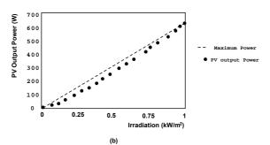
**Figure 4** Results of the MPPT method on PV output power (a) with the proposed MPPT system in operation (b) without the proposed MPPT system, but with the duty cycle adjusted such that the maximum power is produced with solar radiation of 1 kW/m<sup>2</sup> at 25°C.
