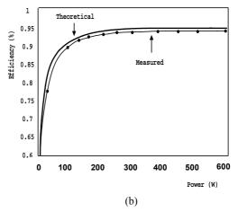
**Figure 3** Theoretical and experimental efficiency of the DC/DC converters designed for (a) the PV panels and (b) the wind generator
