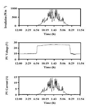
Figure 6 PV array irradiation, voltage and current without MPPT
