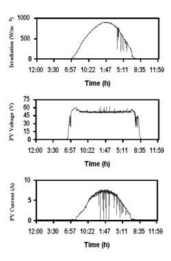
Figure 7 PV array irradiation, voltage and current, when connected to a power grid through an inverter with MPPT
