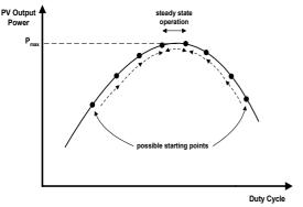
Figure 2 The MPP tracking process
