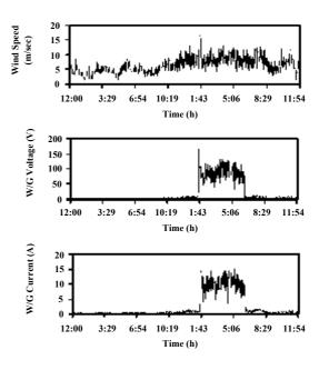
Figure 5 Wind Generator speed, voltage and current
