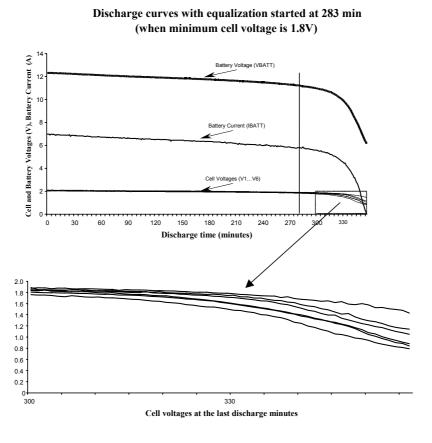
Fig. 3. Experimental discharge curves with equalization started when cell voltage is 1.8V
