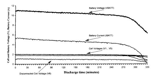
Fig. 4. Experimental discharge curves with one cell fully disconnected.
