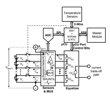
Fig. 2. Block diagram of the proposed Smart Battery Module (SBM).
