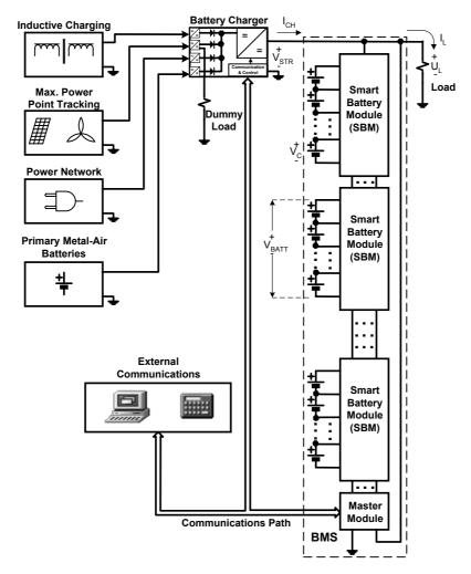
Fig. 1. Block diagram of a typical BMS topology.
