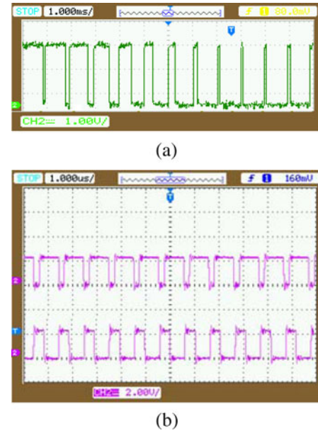
Fig. 8. Oscilloscope measurements of the T_{a+} SPWM control signal: (a) f_c = 1 kHz, f_s = 4 MHz, and M = 0.9 and (b) f_c = 1 MHz, f_s = 32 MHz, and M = 0.5 .
