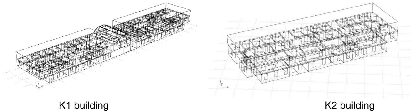
Figure 7. K1 & K2 Building models in ESP-r.
