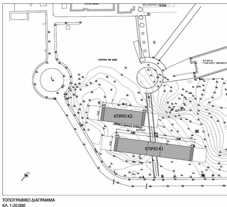
Figure 2. Topographic plan of campus buildings K1 and K2.
