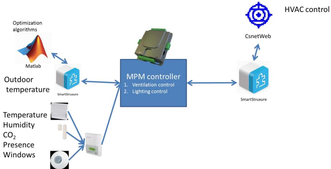
Figure 10. Interconnection of control algorithms local controllers and HVAC-lighting devices.
