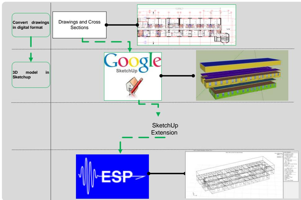
Figure 6. Schematic description of the development of geometry in ESP-r.
