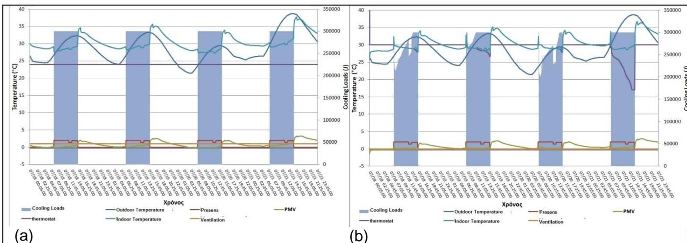
Figure 12. Cooling loads and indoor comfort in a building office with (a) the existing energy management system and (b) the proposed control algorithm during the warmest week of the year.
