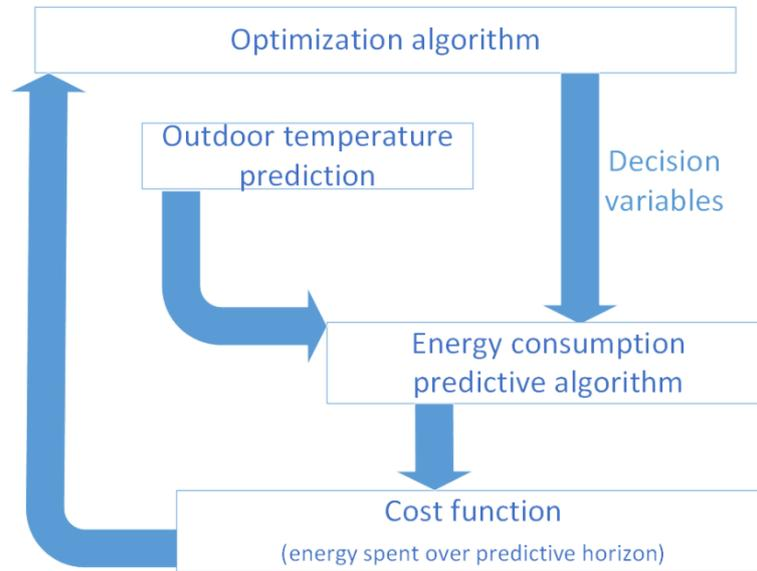
Figure 8. Architecture of optimization algorithms.
