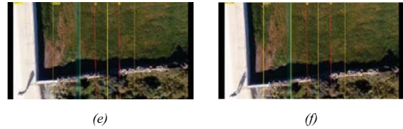
Fig. 8. (a), (b), (c): Correct detection of power lines at subsequent frames - Chania test case – with red the lines / with yellow the ROI boxes, (d), (e), (f): correct fault detection of power lines at subsequent frames - Chania test case.
