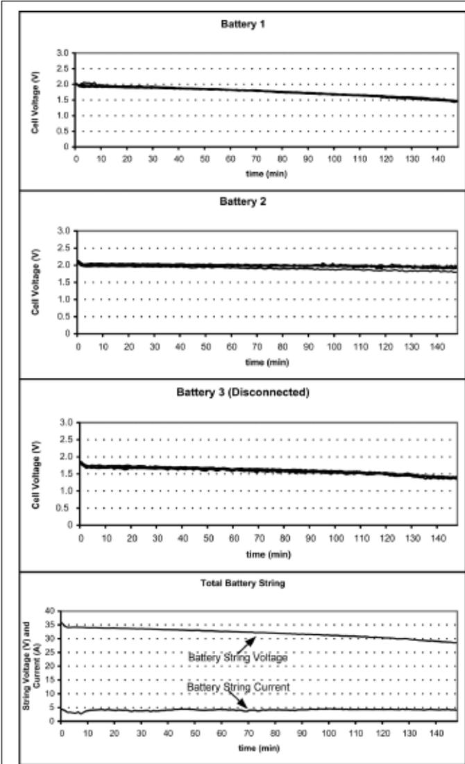
Fig. 7: Experimental discharge curves of a BMS, developed for three 6 cells batteries, with one battery disconnected
