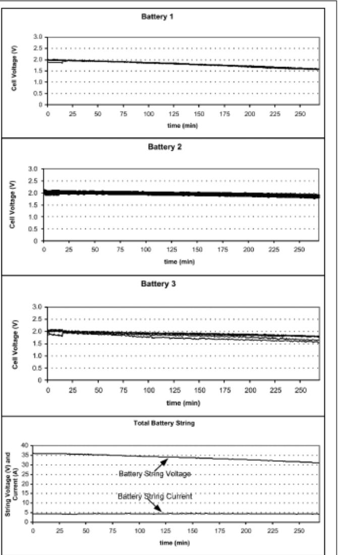
Fig. 8: Experimental discharge curves of a BMS, developed for three 6 cells batteries, with equalization started when minimum cell voltage is 1.8 V
