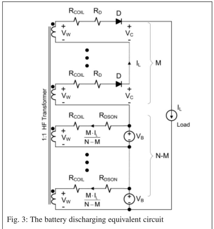
Fig. 3: The battery discharging equivalent circuit
