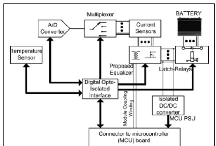
Fig. 4: Block diagram of the experimental Battery Module
