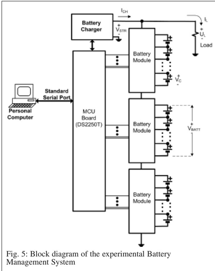
Fig. 5: Block diagram of the experimental Battery Management System
