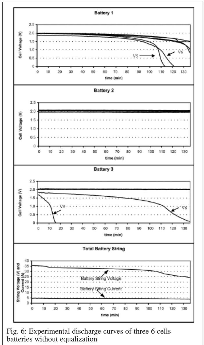
Fig. 6: Experimental discharge curves of three 6 cells batteries without equalization
