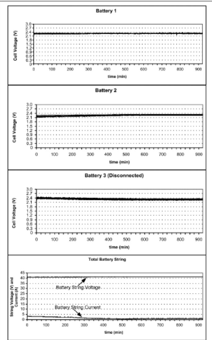
Fig. 9: Experimental bulk charge curves of a BMS developed for three 6 cells batteries, with one battery disconnected
