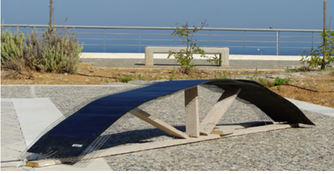
Fig. 7. Flexible PV module experimental setup for the performance evaluation of the proposed global MPPT system (in this example the bending angle is \theta = 90^\circ ).
