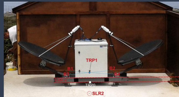
Transponder reference points for the measurements made for Cryosat-2 calibration, using the SLR2 site in Crete, Greece, on 10-May-2013 20:21:40 UTC.
